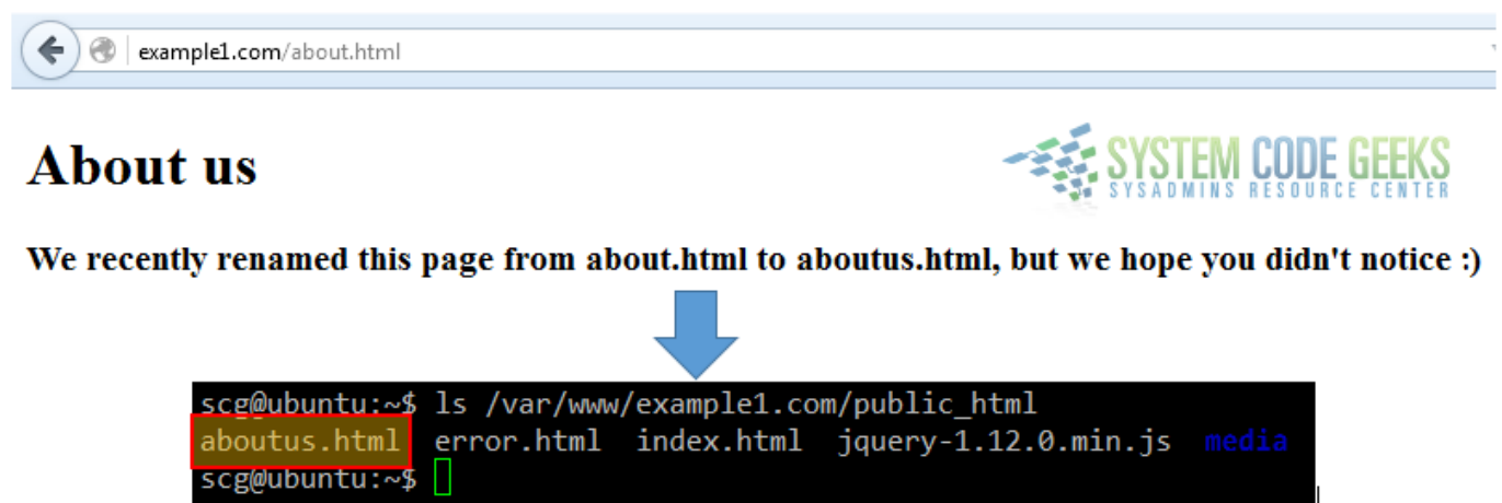
Figure 6.1: Redirecting to a new resource without visible URL change
