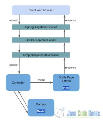
Figure 11.1: grails-architecture
