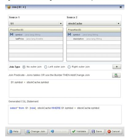
Figure 6–12 Editor Dialog for Oracle CQL Join Operator
