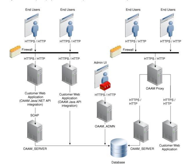
Figure 1–2 Sample deployment scenario for performance and scalability
