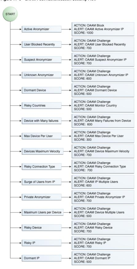
Figure 11–6 OAAM Post Authentication Security Flow
