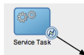
Figure 6–47 The Error Catch Event as a Boundary Event on a Service Task
