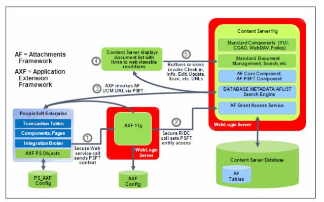
Figure 1–13 System Architecture for an Oracle PeopleSoft Managed Attachments Solution
