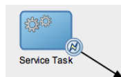
Figure 6–48 The Error Catch Event as a Boundary Event on a Service Task
