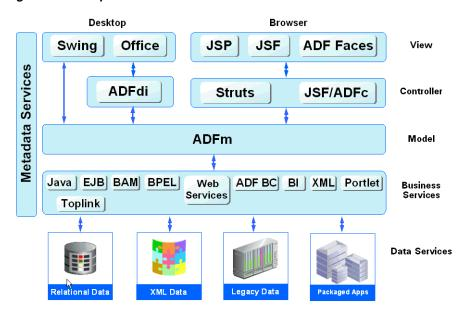
Figure 1–1 Simple Oracle ADF Architecture
