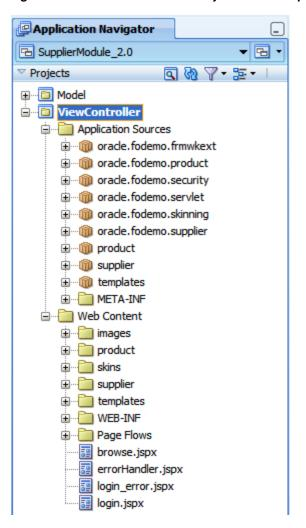
Figure 1–4 The ViewController Project in JDeveloper
