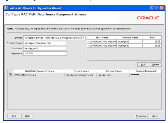
Figure 4-2 Configure RAC Multi Data Source Component Schema Screen
