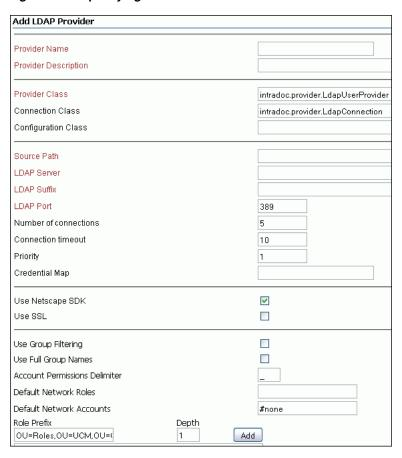
Figure 9–2 Specifying Details of a New LDAP Provider
