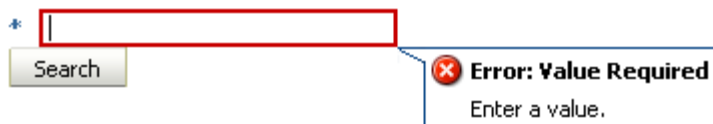
Figure 4-7 Client -side Validation Displays an Error Without a Trip to the Server
