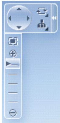
Figure 29–3 Control Panel in Show State
