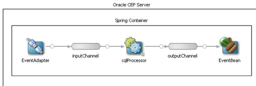
Using Oracle CEP, you can define event adapters for a variety of data sources including JMS, relational database tables, and files in the local filesystem. You can connect multiple input channels to an Oracle CQL processor and you can connect an Oracle CQL processor to multiple output channels. You can connect an output channel to another Oracle CQL processor, to an adapter, to a cache, or an event Bean.
