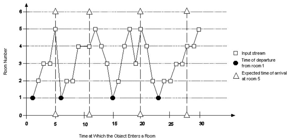
[Example 15–22](#) shows query `q` on stream `S` (with schema `c1` integer representing room number) that detects these non-events. Each time the object fails to reach room 5 within 5 minutes of leaving room 1, the query returns the time of departure from room 1.
