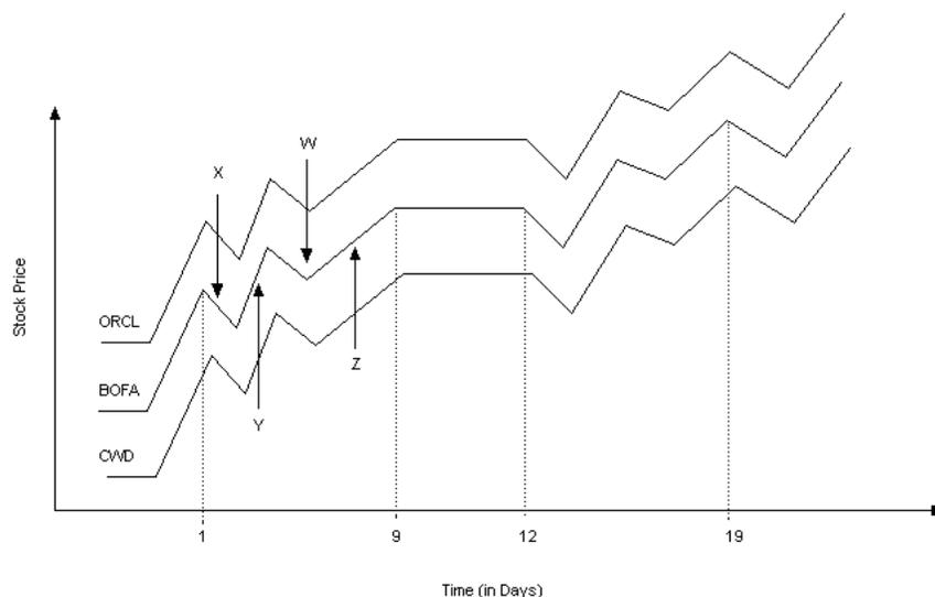
**Example 15–18** shows a query `q` on stream `S2` with schema `c1` index number (or time) and `c2` stock price. This query detects double bottom patterns on the incoming stock trades using the `PATTERN` clause (`A W+ X+ Y+ Z+`). The correlation names in this clause are:
