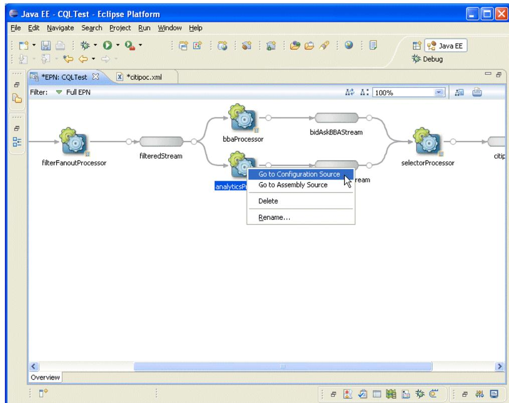
The EPN Editor opens the corresponding component configuration file for this processor and positions the cursor in the appropriate `processor` element as [Figure 14–2](#) shows.
