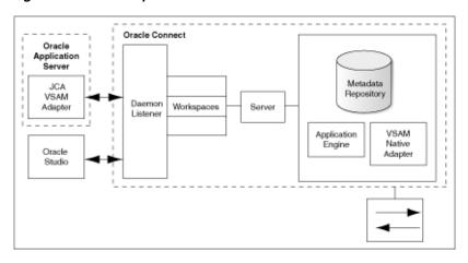
Figure 1–1 The Adapter Architecture
