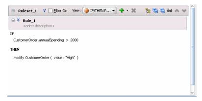
At runtime, when this rule is processed the Rules Engine checks the facts against rule pattern tests that you define to find matching facts. For this sample rule, Rule\_1, when a fact matches the Rules Engine modifies the fact and then modifies the value property to "High".
