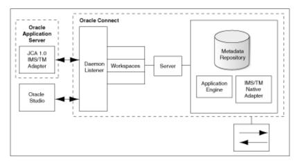
Figure 1–1 Adapter Architecture
