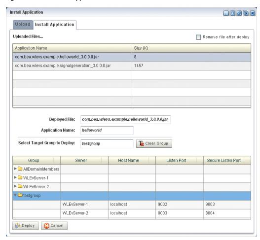
Figure 5–3 The Install Application Screen: Multi-Server Domain
