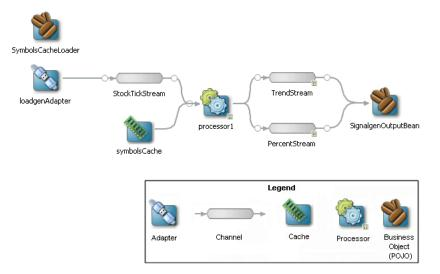
Figure 3–81 The Signal Generation Example Event Processing Network
