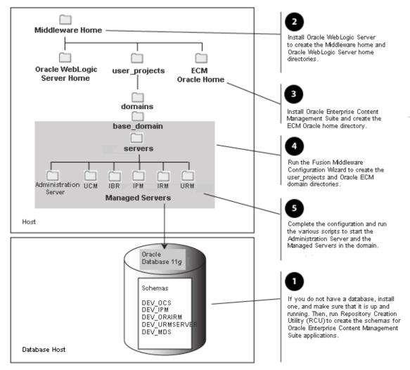
The topology in Figure 1–2 includes multiple applications configured on the same host in one Oracle WebLogic Server domain that includes only Oracle Enterprise Content Management Suite applications. The schemas for the applications are in the same database.
