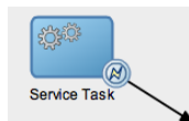
Figure 6–41 The Error Catch Event as a Boundary Event on a Service Task
