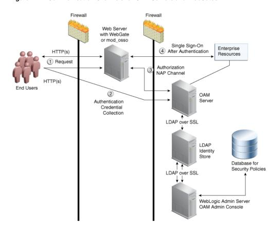
Figure E-1 Communication Channels for OAM Servers and WebGates
