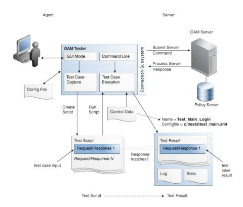
Figure 10-2 User Interactions with the Access Tester
