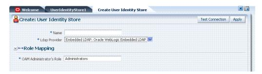
Figure 3–2 illustrates a completed user identity store registration page in the Administration Console. With the exception of the Embedded LDAP store, all registrations require the same type of information regardless of the LDAP directory server you are registering. A Test Connection button appears at the top of this page. By default, the embedded LDAP store is set as the Primary user identity store. If a data source is not set as primary, the Set As Primary button is available.
