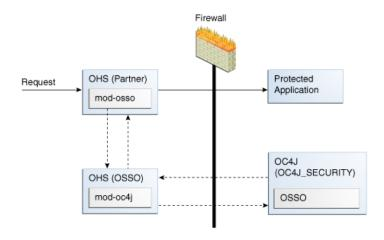
Figure B-2 Pre-Upgrade Sample OSSO 10g with Front-End Proxy
