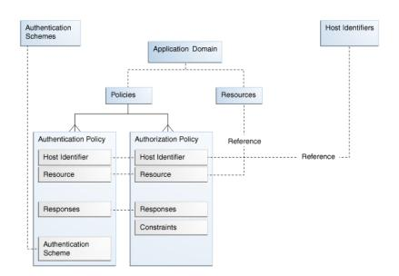
Figure 9-1 Application-Specific Components of the OAM Policy Model
