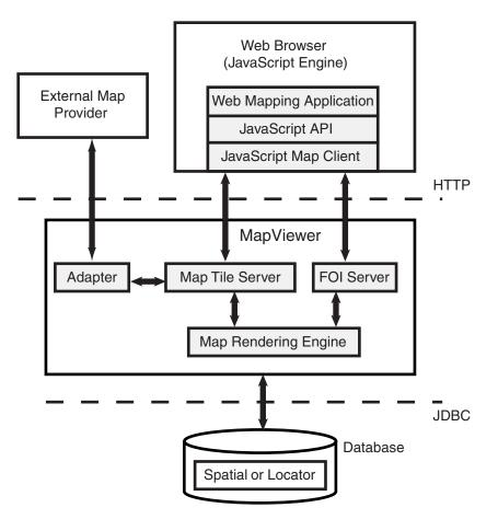
Figure 8–1 Architecture for Oracle Maps Applications
