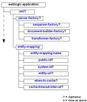
Figure 8–1 Sub-Elements of the <xml> Element in weblogic-application.xml
