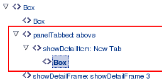
Figure 17–22 Tab Component in Source View
