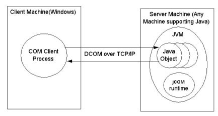
The Java code in the JVM must call com.bea.jcom.Jvm.register(<jvm id>), where <jvm id> is the id of the JVM as defined in regjvm.
