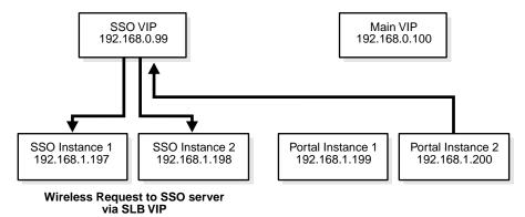
Figure A-3 Request Routing to the OracleAS Single Sign-On Server Load Balancer
