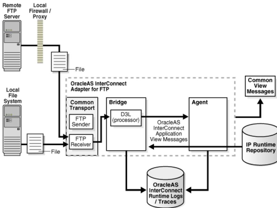
Figure 1-2 shows the data flow of outgoing messages from OracleAS Integration InterConnect to the remote FTP Server.
