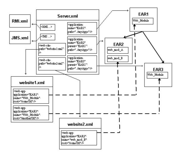
Figure 5–1 Mappings from the server.xml File
