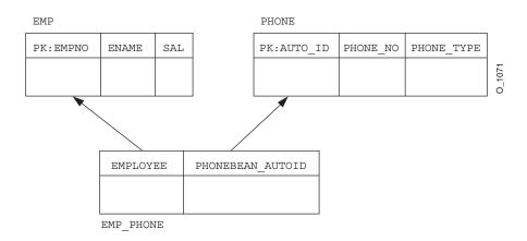
Figure 6–18 Explicit Mapping for One-to-Many Unidirectional Bean Relationship
