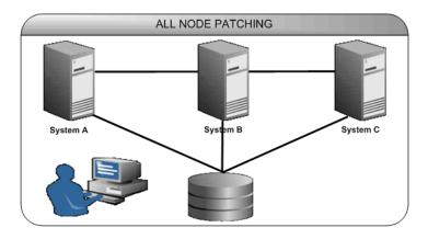
Systems A, B, and C are nodes in this cluster. When you perform All Node Patching in this cluster, you bring down systems A, B, and C, apply patches to all these nodes, then bring systems A, B, and C back up again.
