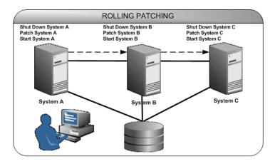
When you perform Rolling Patching in this cluster, the patches are applied in a rolling fashion. You initially bring down system A, apply a patch to it, then bring it back up. You do the same thing for systems B and C.
