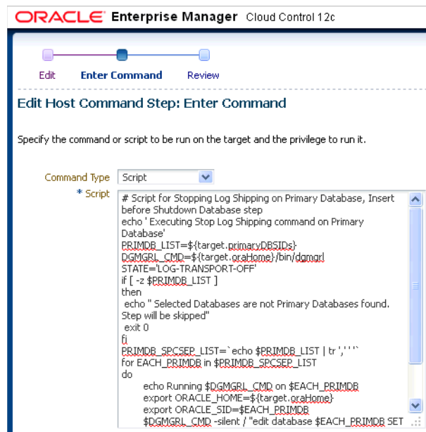
Figure 24–17 Adding a Script for Stopping the Log Shipping
