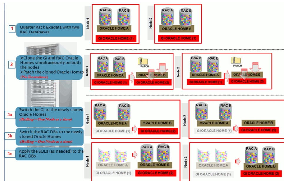
Figure 24–13 Out Of Place Patching Of Clusters
