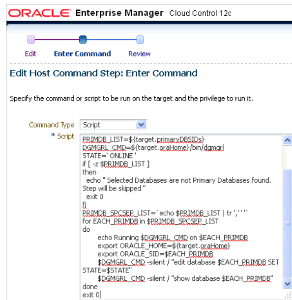
Figure 24–18 Adding a Script for Starting the Log Shipping
