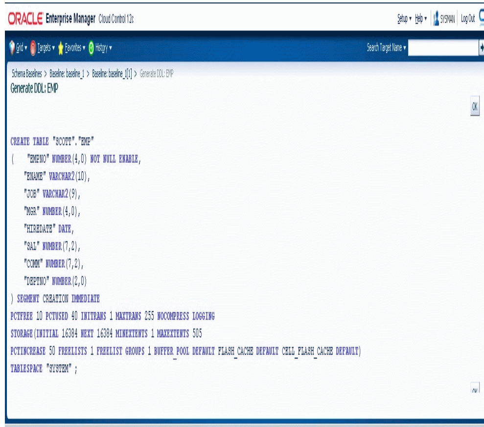
Figure 28–3 DDL Generated for a Selected Baseline Object
