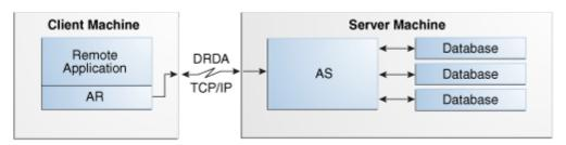
The application uses the AR to communicate with an AS, which in turn communicates with the database. In this configuration, applications are indirectly aware of the network because the AR connects to the network. The application does not require direct knowledge of the network connectivity.
