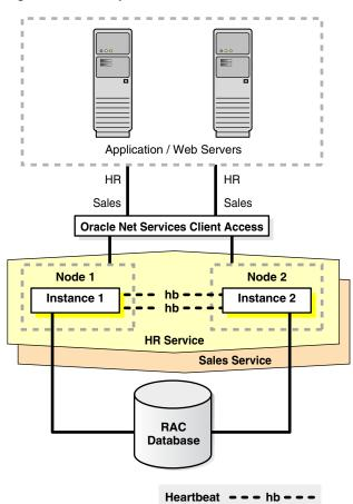
Figure 12–9 Nonpartitioned Oracle RAC Instances
