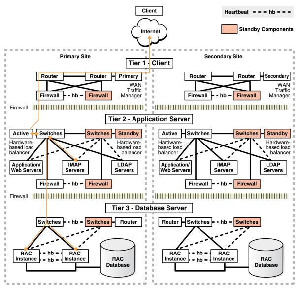
Figure 12–3 illustrates the network routes after site failover. Client or application requests enter the secondary site at the client tier and follow the same path on the secondary site that they followed on the primary site.
