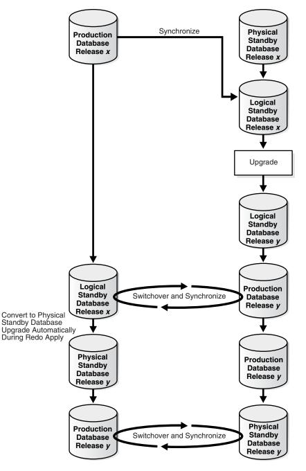
Figure 13–1 Using a Transient Logical Standby Database for Database Rolling Upgrade
