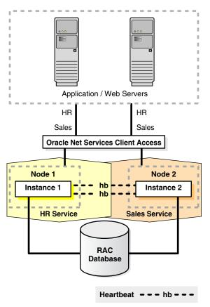
Figure 12–7 Partitioned Two-Node Oracle RAC Database
