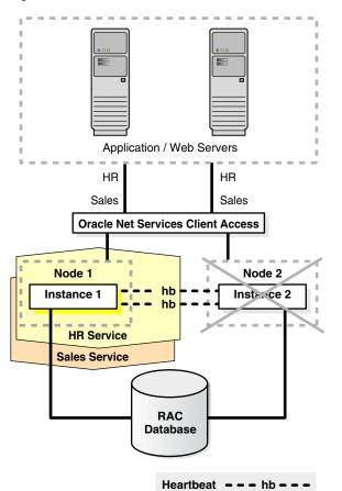
Figure 12–8 Oracle RAC Instance Failover in a Partitioned Database
