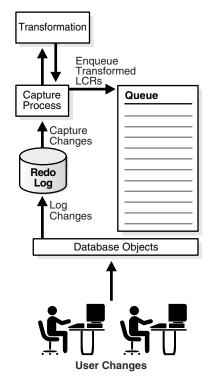
Figure 6–1 Transformation During Capture by a Capture Process
