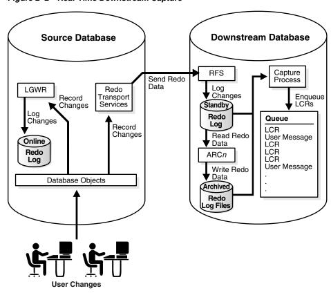
Figure 2–2 Real-Time Downstream Capture
