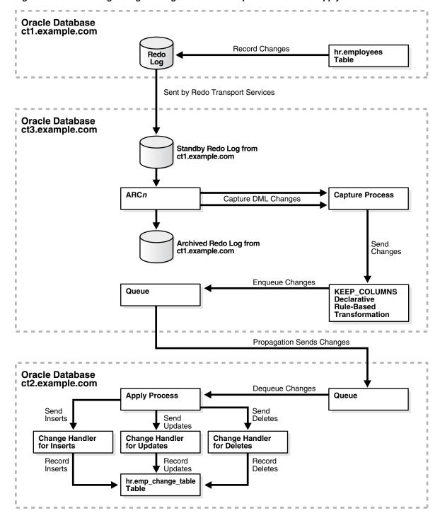
Figure 20–4 Recording Changes Using Downstream Capture and Remote Apply
