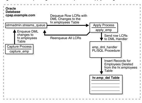
Figure 1–6 Sample Single Database Capture and Apply Configuration
