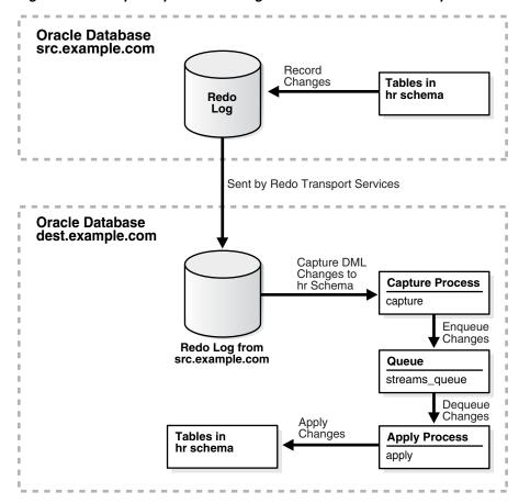
Figure 1–3 Sample Replication Configuration with Downstream Capture
