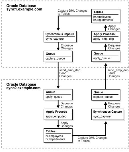
Figure 1–4 Sample Replication Configuration with Synchronous Captures
