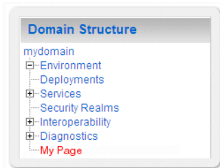
Figure 6-3 Append a Node to the Root of the Existing Tree
