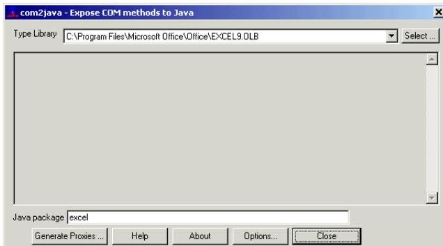
2. Select the appropriate type library in the top field, and fill in the Java package text box with the name of the package to contain the generated files. The `com2java` tool will remember the last package name you specified for a particular type library.
