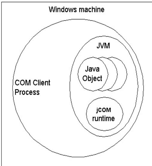
The JVM need not call `com.bea.jcom.Jvm.register()` or be started as an extra process to the client.
