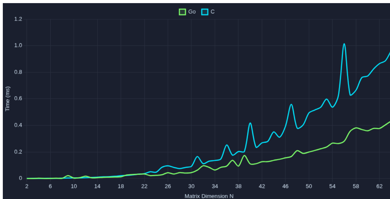
Figure 6. Go vs C head-to-head. Go generally outperforms C. N=9 Go spike = runtime warm-up. N=40, N=56 C spikes = cache boundary.
