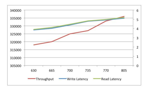
Couchbase Server did not exceed the maximum latency of 5ms until 805 concurrent clients. These last tests indicate Couchbase Server can reach up to 4.5x the throughput of MongoDB while maintaining latency of 5ms or less. Assuming MongoDB scales linearly, it would have required 4-5x the number of nodes to provide the same performance as Couchbase Server.
