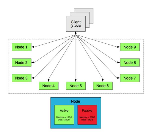
The Couchbase Server topology is simple. Each client responsible for running YCSB communicated directly with the Couchbase Server nodes. The range of clients that Couchbase Server was able to handle before exceeding the 5ms latency threshold was 2-23.
