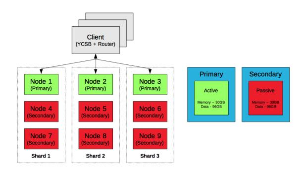
This image shows the MongoDB topology for the benchmark. For running the benchmark, we had YCSB located on the same node as the router. Each client/router node communicates via the configuration server nodes, which contains metadata pertaining to each shard. The range of clients that MongoDB was able to handle before exceeding the 5ms latency threshold was 2 – 7.
