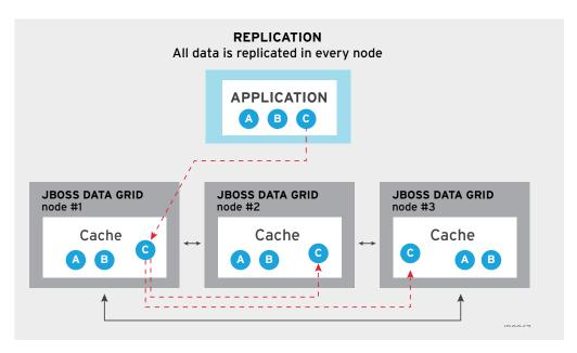
In the replicated configuration, the same exact data exists on all nodes of the clustered cache. This can be ideal for applications that require extremely high fault tolerance, and real-time read access by multiple applications. The amount of data available for in-memory processing is limited by the amount of memory on each server.
